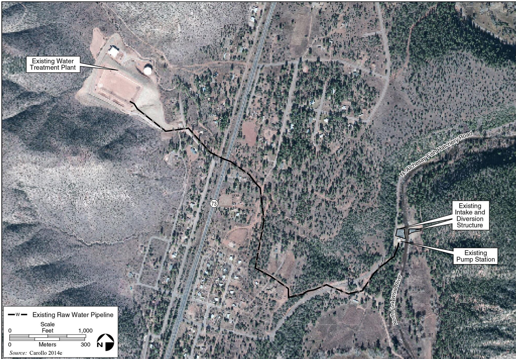
Figure 2.3-1. Existing North Fork Intake Structure and White River Surface Water Treatment Plant
